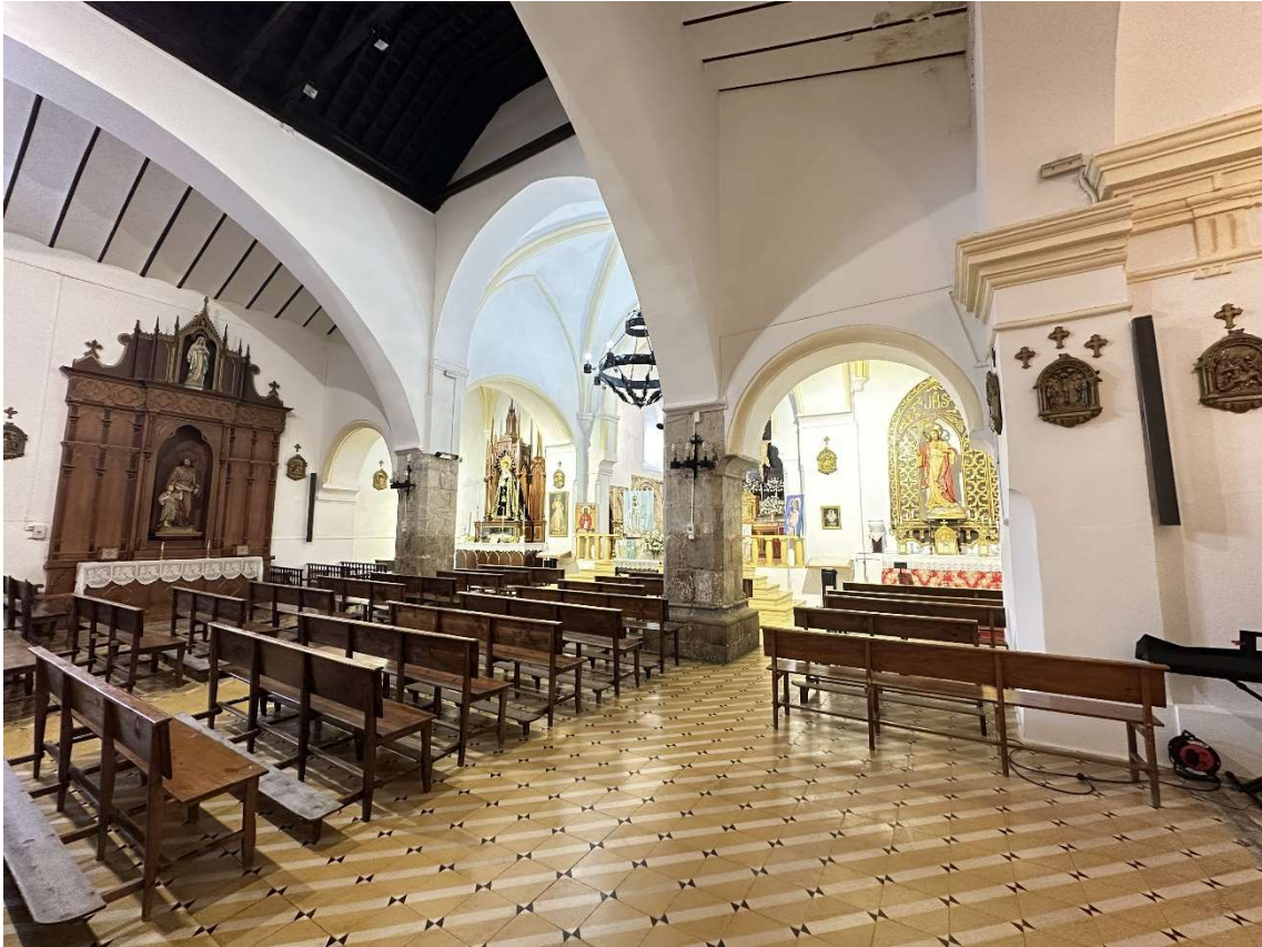
Rectangular floor plan with three naves separated by thick columns and attached side chapels. © ARZOBISPADO DE TOLEDO. TOLEDO. ESPAÑA
